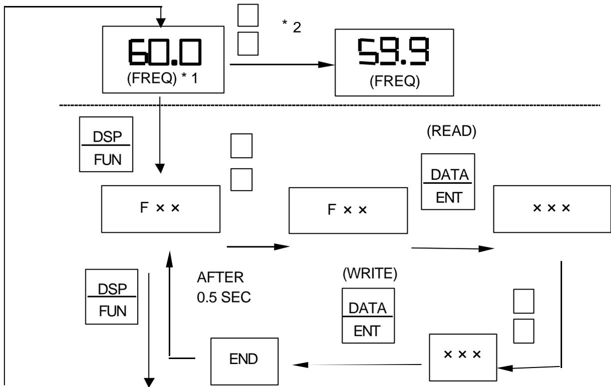
Note 1: Displayed setting of frequency when stopped. Display output frequency when running.
