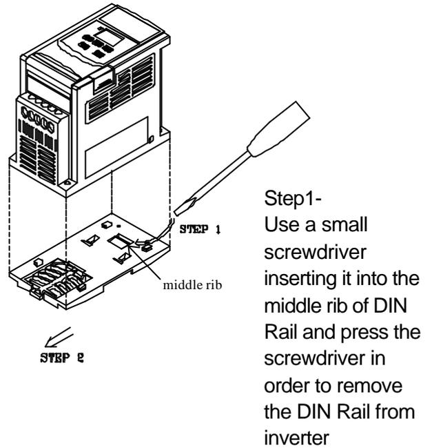
Step1- Use a small screwdriver inserting it into the middle rib of DIN Rail and press the screwdriver in order to remove the DIN Rail from inverter
