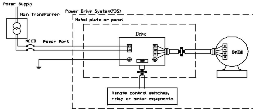
When the distance between the inverter and motor is longer than 100 meters, cable wire should be carefully chosen to reduce the wiring resistance below 3% and the voltage drop  $(V) = 3 \times \text{Wire resistance } (\Omega/\text{km}) \times \text{wire length (m)} \times \text{current} \times 10^{-3}$
