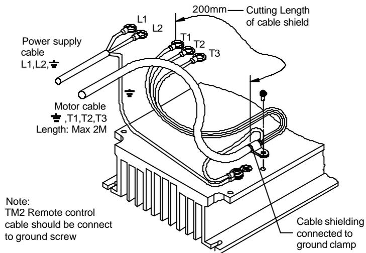
E2-1P2~201- -N4S (WITH SWITCH TYPE ) EMC MOUNTING & CONNECTIONS :
