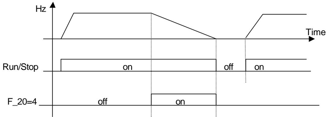
5. F\_19, F\_20 = 5: Auto Reset when inverter faults.
