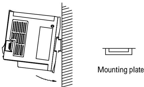
First place the groove on the back of module on the upper edge of din rail, and then push the module down to lock up position. Finally press the mounting plate upward into module.
