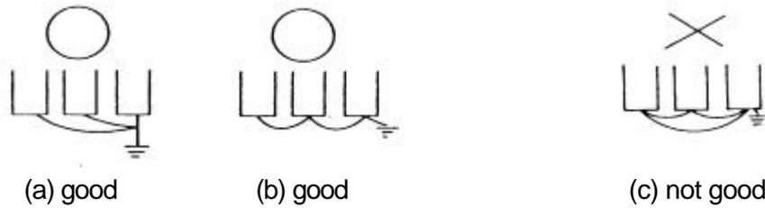
(D) Wire specification, apply appropriate wire with correct diameter for primary power circuitry and control circuitry in accordance with electricity regulations.
