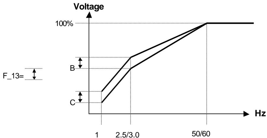
**NOTE:** When  $F_{13} = 0$ , the torque boost function is disabled.
