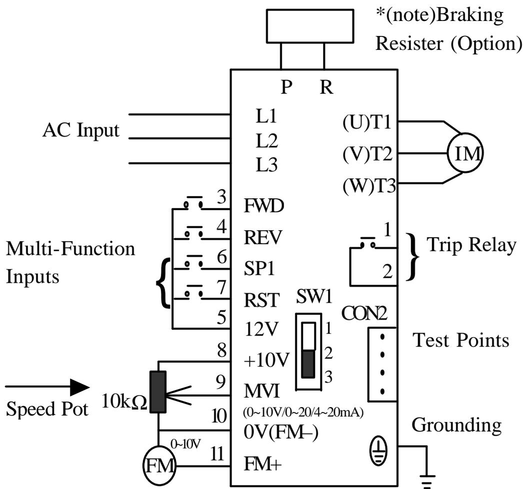
Wire Terminations to the Inverter must be made with either UL listed field wiring lugs or UL listed crimp type ring terminals.
